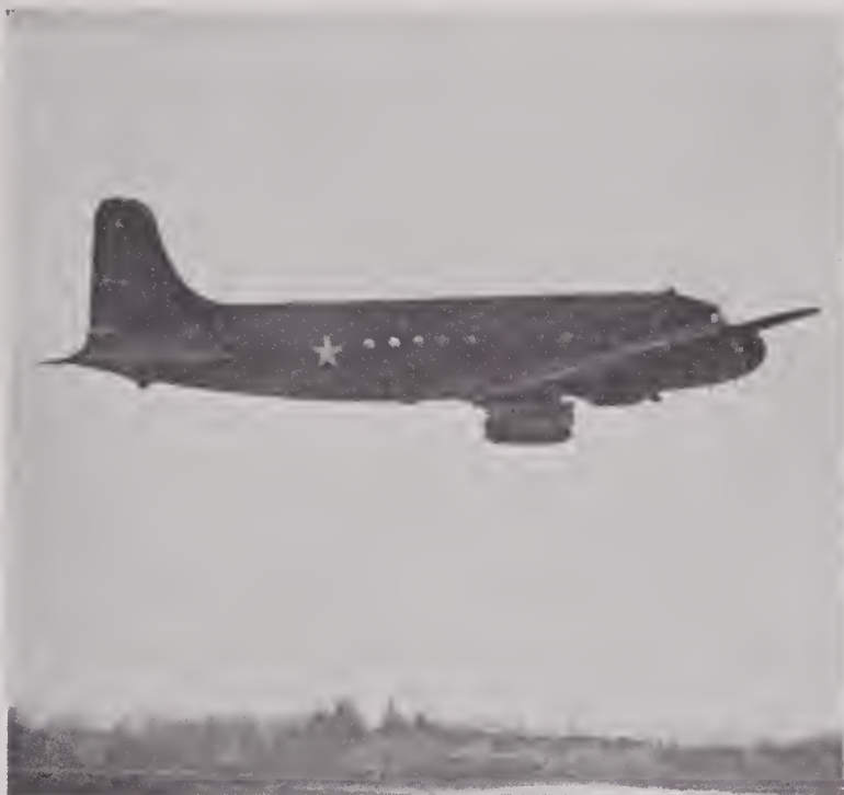
FIGURE 37. C-54 taking off at Wright Field, Dayton, Ohio, with T-15 Weasel secured for experimental parachute drop.
